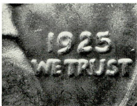
Counterfeit 1925 Fort Vancouver half dollar. Rounded date and lettering. Numerous raised lumps of metal.
