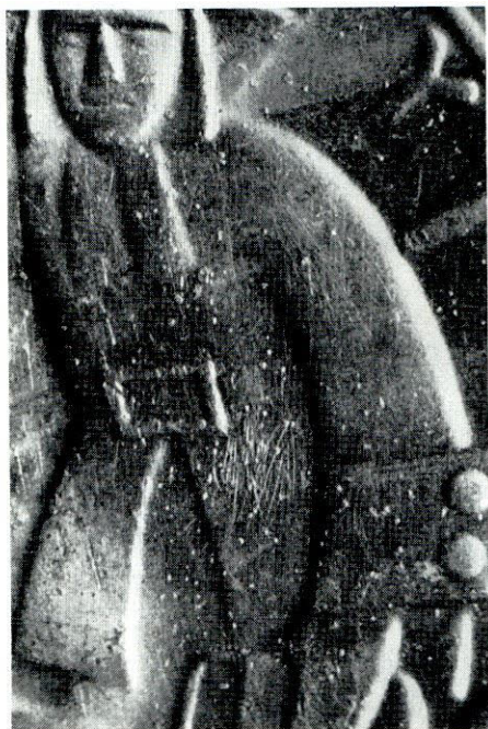
Die polish marks and die rust on obverse figure of Roger Williams.
