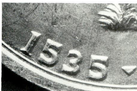
Counterfeit 1935 Spanish Trail half dollar. Rounded numerals in 1535, no die polish lines.
