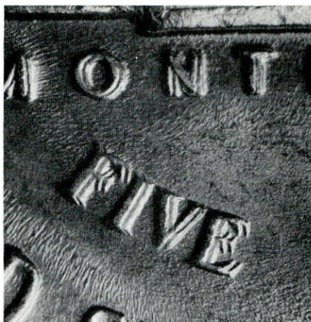
1939 five cents: Doubled die reverse. Letters display a raised, rounded effect and distinct notches on serifs.
