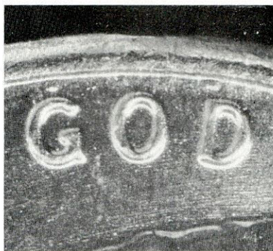
Doubling is evident on IN GOD WE TRUST, especially inside the upper portion of GOD.
