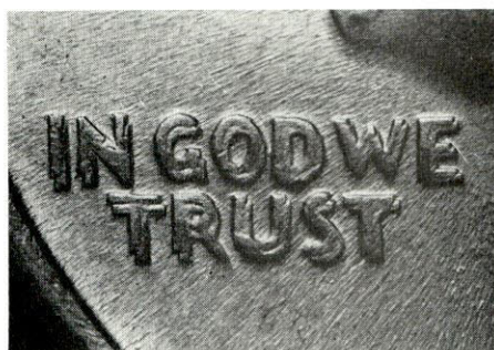
1934 quarter: Doubled die obverse. Doubled motto was caused during the hubbing process and is duplicated on every planchet struck with this die.
