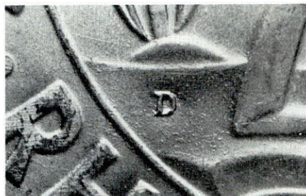
Heavy die rust around characteristically sharp mintmark.
