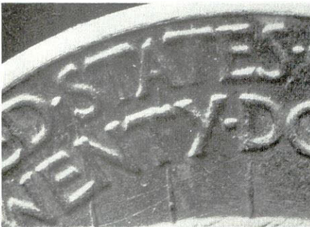
Raised lines below TWENTY and between STA of STATES.
