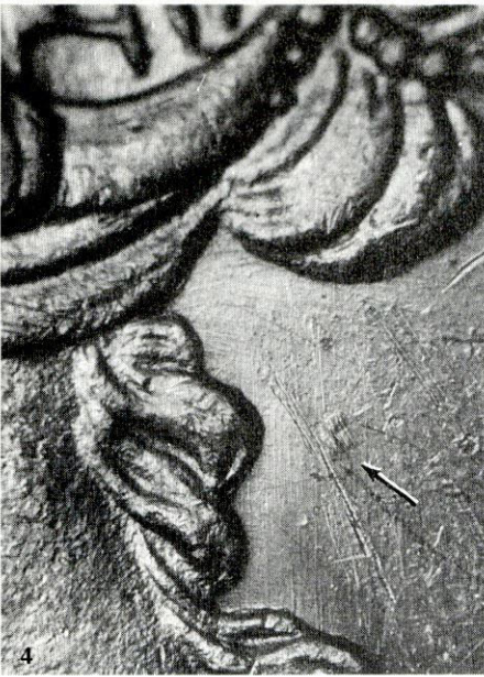
4 Tool marks in field to right of hair strand at back of Liberty's neck, the result of an attempt to correct a depression in the die.
