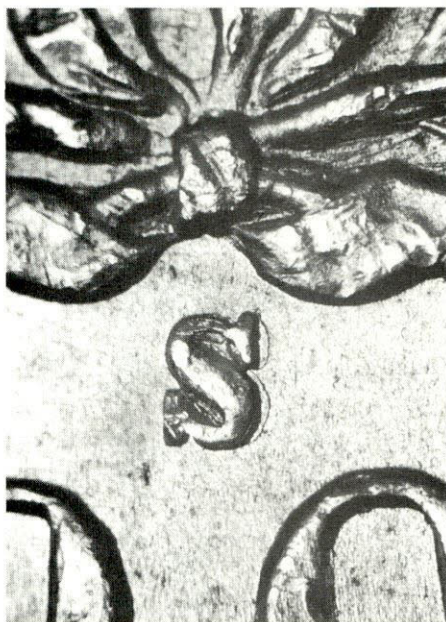
1881-S Morgan dollar: Machine doubling on mintmark. Excess machine wear allows die to shift sideways during or immediately after impact.
