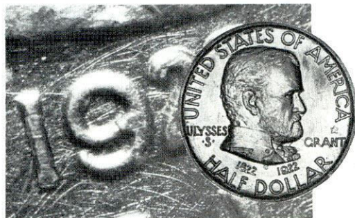
Commemorative coins often show extensive die polishing. An excellent example is the 1922 Grant commemorative half dollar with star, which features heavy die polish marks around the date.
