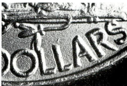
Counterfeit: Raised lumps of metal through DOLLARS on reverse.
