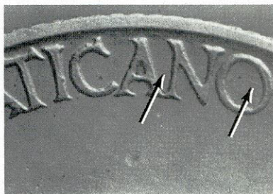
Raised lines of metal run through AN and O of VATICANO.
