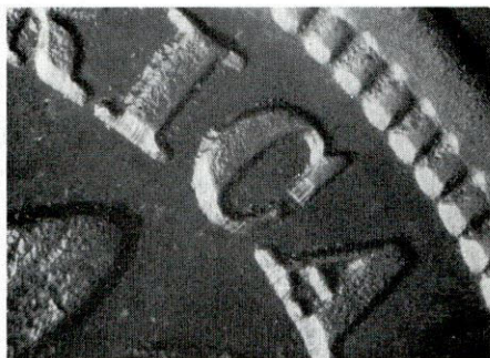
More granular characteristics of the EDM counterfeit on this 1863 cent.
