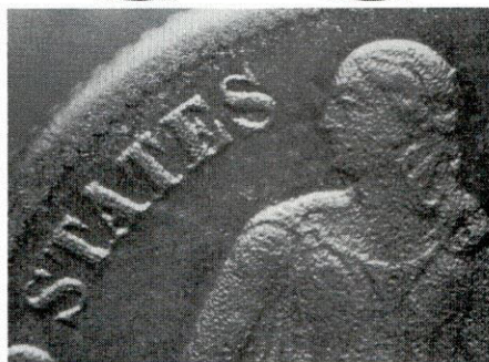
Rough, granular letters and devices on an EDM counterfeit 1866 dime.
