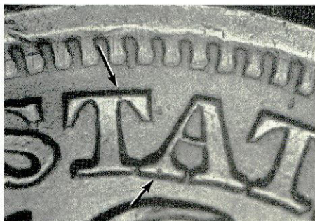
Pits in upper horizontal bar of first T and in the left base of A in STATES.
