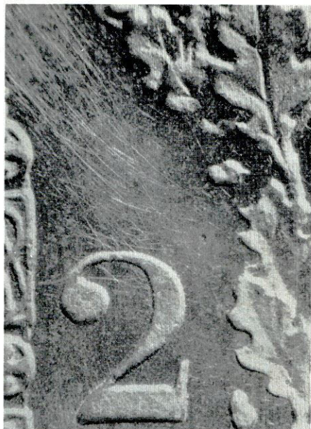
1885-R 2-lire, counterfeit reverse: weak details, raised tool marks in field.
